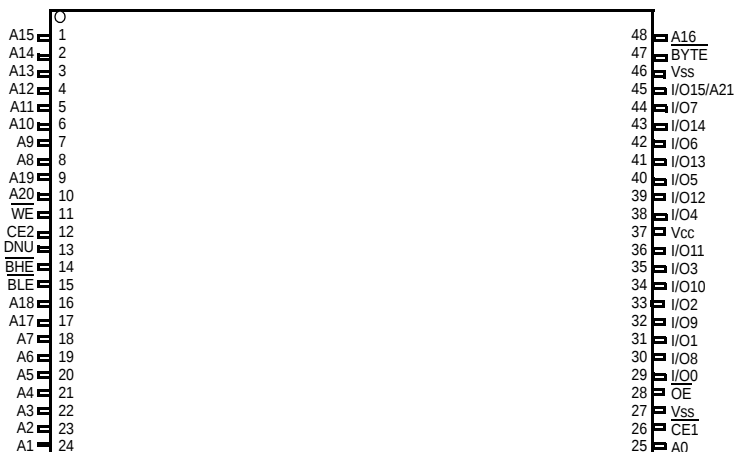
Figure 1. 48-pin TSOP I pinout (Front View) [1, 2]
