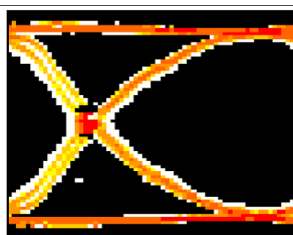
Figure 11. Internal Eye Monitor Hit Density Plot
