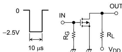
$V_{DD} = -10 \text{ V}$
