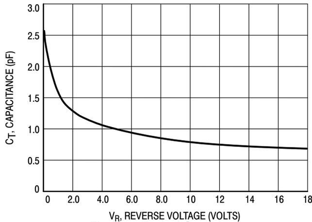
Figure 4. Typical Capacitance
