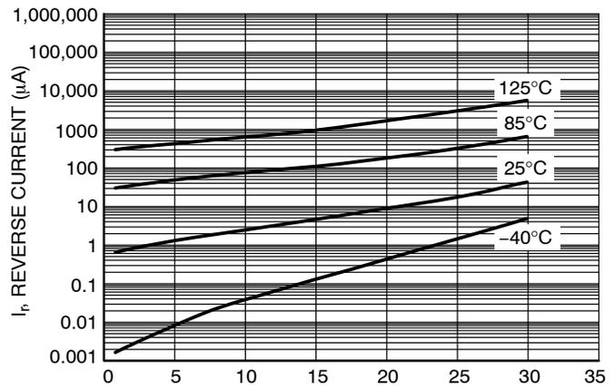
**Figure 2. Leakage Current**
