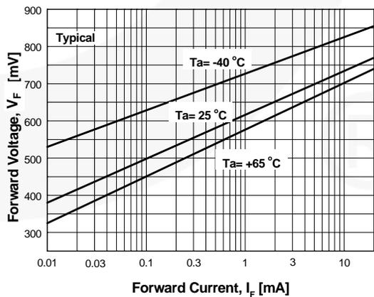
Figure 6. Forward Voltage vs. Ambient Temperature
