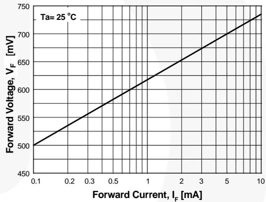
Figure 4. Forward Voltage vs. Forward Current
