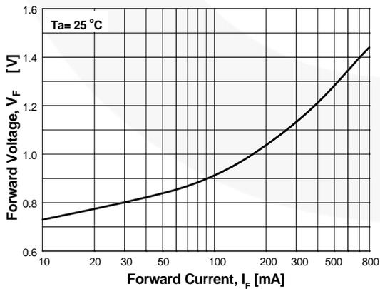
Figure 5. Forward Voltage vs. Forward Current
