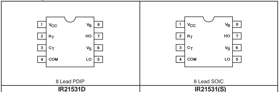
NOTE: The IR21531D is offered in 8 lead PDIP only.
