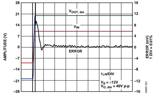
Figure 31. Settling Time,  $V_S = \pm 12 V$
