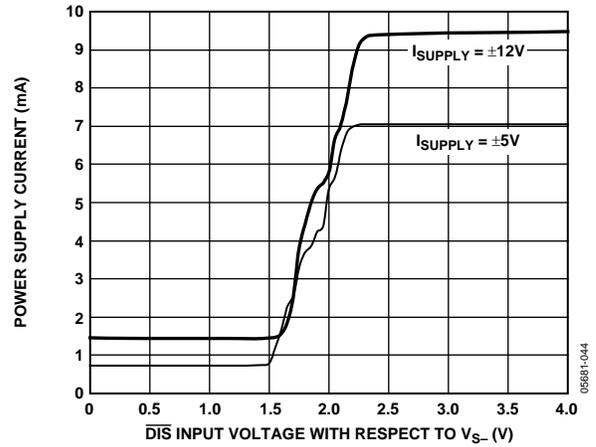
Figure 37. Power Supply Current vs. Disable Input Voltage
