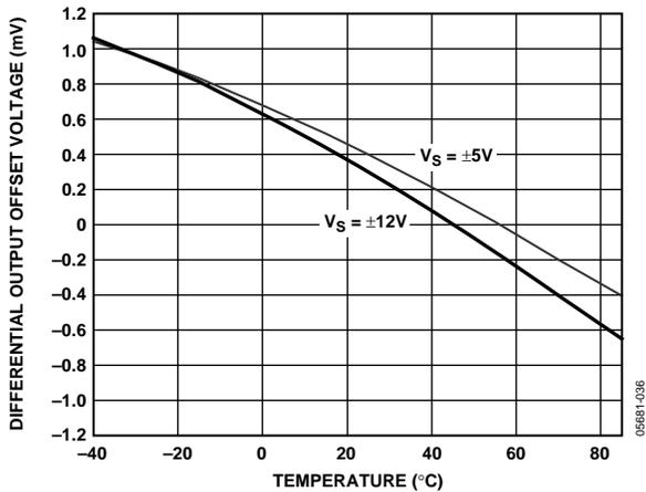
Figure 30. Differential Output Offset Voltage vs. Temperature
