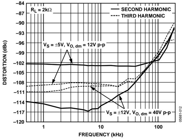
Figure 17. Harmonic Distortion for Various Power Supplies
