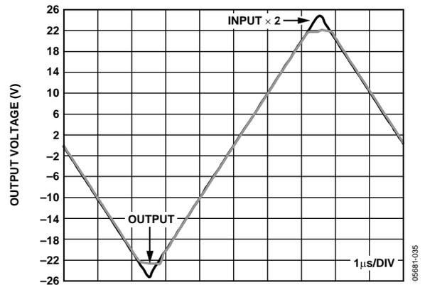
Figure 32. Input Overdrive Recovery,  $V_S = \pm 12 V$
