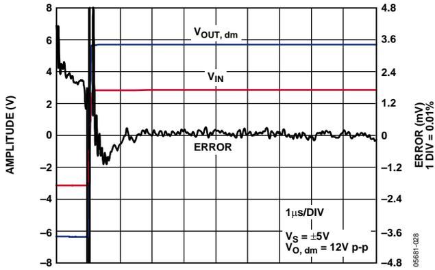
Figure 28. Settling Time,  $V_S = \pm 5 V$
