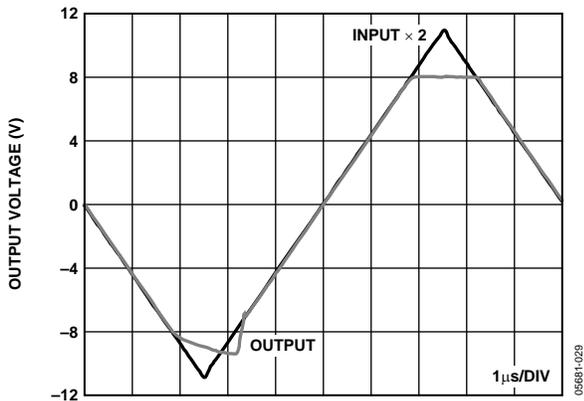
Figure 29. Input Overdrive Recovery,  $V_S = \pm 5 V$
