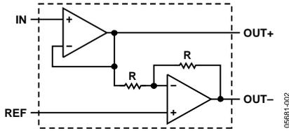
Figure 41. Functional Diagram
