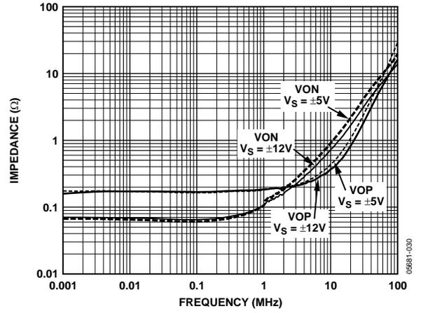
Figure 21. Single-Ended Output Impedance vs. Frequency and Supplies
